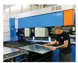
The BCe Smart with its innovative servo-electric bending technology is the optimal solution for medium production volumes as well as for low volume or lean production. It guarantees precision and repeatability with a considerable reduction of maintenance costs.
