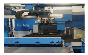
The 4 kW fiber source and the punching unit with over 300 tools allow the Combi Genius to process sheet metal up to 8 mm.
