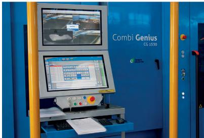
A Prima Power Combi Genius 1530 punching/laser cutting machine with a 4 kW fiber laser and an LSR6 loading/unloading and stacking robot is connected to the Night Train.
