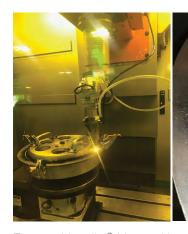
Two part Hastalloy® X assembly pictured left during the automated welding process. The new LASERDYNE 430 system precisely controls the power, position, and focus for a perfect end result without cracks or voids in the weld structure.
