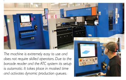
With the BCe Smart, managing the entire production process is easy and efficient, with the Open numerical control by Prima Electro, the Tulus operator interface, and the Master Bend Cam programming system. The machine is also prearranged to be integrated with robots for the automatic loading and unloading.
