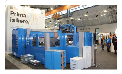
Making its world premiere at Blechexpo was Prima Power's new bending solution, the eP Genius 1030, consisting of the integration of a servo-electric press brake eP-1030 with an automatic tool change storage. The result is a faster and more versatile and reliable bending system, especially designed for minimum batches. This makes it possible to reliably estimate the machine set-up and short cycle times which are imperative to gain a higher market competitiveness.
