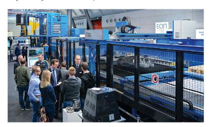
In Stuttgart, Prima Power also displayed the high-performance **Laser Genius 1530** fiber laser machine with 10kW laser, featuring new cutting strategies allowing top performance of cutting speed, piercing time, and reduction of gas consumption. The machine was showcased with the Combo Tower Laser, a flexible storage system integrating loading and unloading for the optimal solution in lights-out production.
