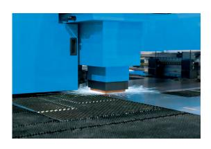
two drop doors are provided as standard; 300 mm x 400 mm for quicker sorting and 800 mm x 800 mm for larger parts. New brushes on the chute top prevent scratches. From the drop door, the parts are transferred by conveyor to the side of the machine to be unloaded manually or forwarded with different conveyor and sorting solutions.
