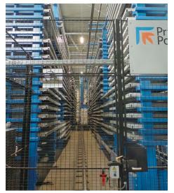
The Night Train Flexible Manufacturing System allows optimal management of raw materials, semi-finished products and scraps, allowing a single operator to control all production.
