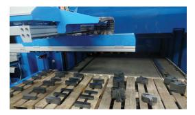
Prima Power's LST sorting system is able to palletize even pieces with complex geometries, thus allowing a fully automated production flow.
